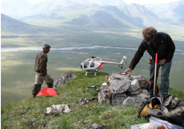
Chuck & Daryl placing a cadastral monument above the Anaktuvuk River
